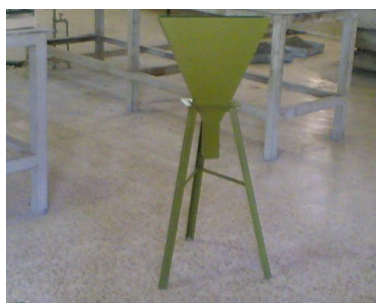
Figure (4): V-funnel apparatus
