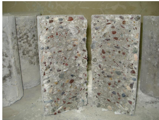
Figure (12): Linear Failure of cylinder
